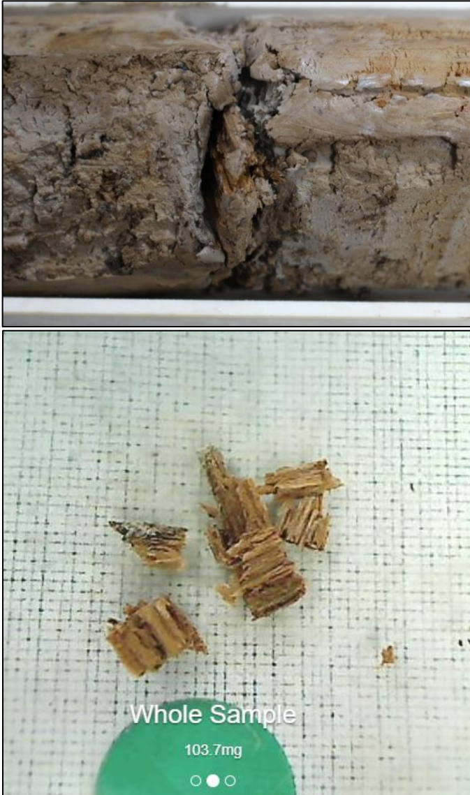
Figure 5. Top: Wood fragment in the C4 core. Bottom: Sample submitted for radiocarbon dating (photo courtesy of Beta Analytic, Inc.).
