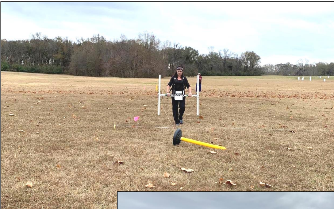
Figure 3. UAB student Marsha Holley running the magnetic gradiometer in the plaza at Poverty Point WHS under the watchful eye of Mike Hargrave. Photo courtesy of Rinita Dalan.
