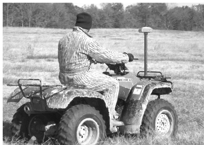
Figure 1: Lee Overby using the NRCS 4-wheeler with onboard GPS to map the topography of the plaza and ridges at Poverty Point SHS.
