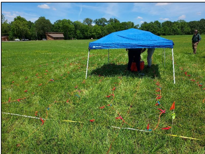
Figure 4. Transects of electrodes and cable for 2.5D modeling. Jimmy Adcock (left) and Rinita Dalan (right) in background.
