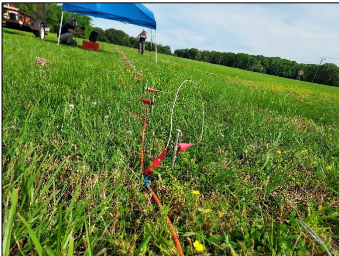
Figure 4. Transects of electrodes and cable for 2.5D modeling. Jimmy Adcock (left) and Rinita Dalan (right) in background.
