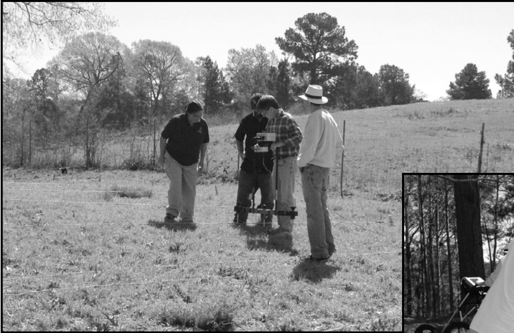
Above- Everyone helped with the resistivity survey since it is the most time-consuming of all the geophysical survey techniques. Readings are taken every meter by poking the probes into the ground and pushing a button. (left to right, Rhonda Gauthier, Charles Aston, Jeff Girard, and Jami Lockhart). Right- Jeff Williams and Boogie Windsor take their turn with the resistivity meter. Below- The resistivity meter gave the best results. A large rectangular anomaly might be the mission church.
