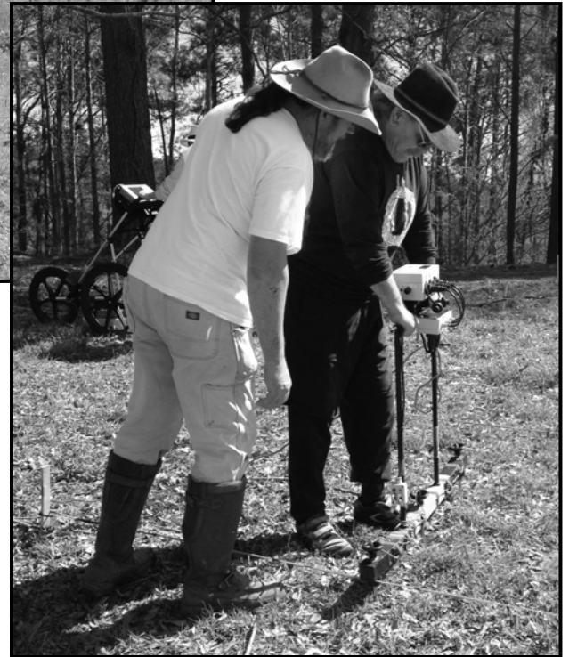
Above- Everyone helped with the resistivity survey since it is the most time-consuming of all the geophysical survey techniques. Readings are taken every meter by poking the probes into the ground and pushing a button. (left to right, Rhonda Gauthier, Charles Aston, Jeff Girard, and Jami Lockhart). Right- Jeff Williams and Boogie Windsor take their turn with the resistivity meter. Below- The resistivity meter gave the best results. A large rectangular anomaly might be the mission church.
